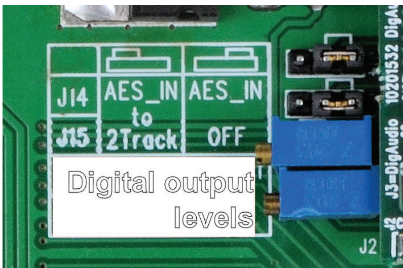
Close up of jumper settings
