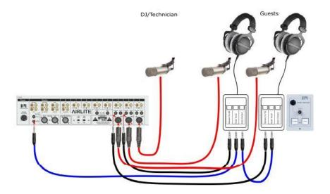
Practical wiring diagram for the AIRLITE mixer
